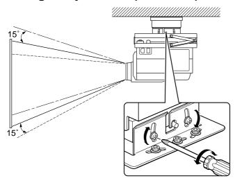
4 Center the projected image on the screen vertically and then fasten the projector securely by tightening the bolts.
