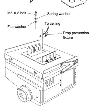
4 Attach the drop prevention fixture to the ceiling using the same procedure as described in items 1 - 3.
