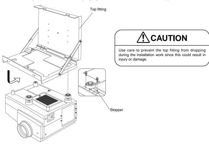
4 Firmly tighten the accessory screw (M8 × 15mm) and the two DLA-G10U/E legs.
