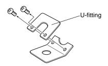
**2** Attach a drop prevention chain or wire to the U-fitting and fasten firmly with a screw.
