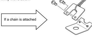
Mount the drop prevention fixture on the ceiling mount.
